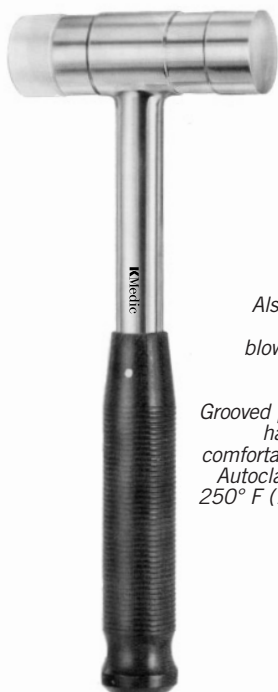
REPROCUSSION FREE Mallet KM 46-690 11½" weight: 1 lb. 5 oz. (600 grams) head weight: 10 oz. (285 grams) head diameter: 32mm dead blow mallet with phenolic handle, one nylon cap and one stainless steel side
