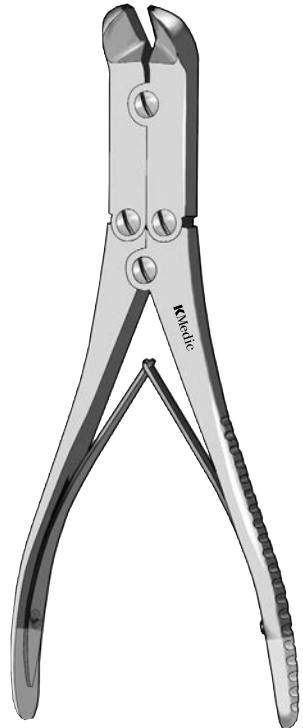
DOUBLE ACTION WIRE CUTTER KM 46-624 8 1/2" angled, side cutting with carbide inserts maximum capacity 3/32" (2.4mm)
