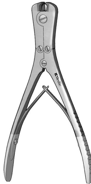
FLUSH WIRE CUTTER KM 46-631 7" front and side cutting with carbide inserts, double action maximum capacity .062" (1.6mm)
