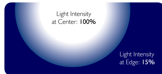
Current Xenon Fiber Optic Headlights Light Distribution
